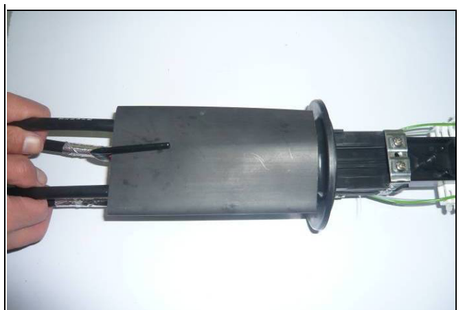
(13) Usage of branch folk: when heating the oval entry port, folk the heat-shrinkable tube to separate the two cables and heat-shrink it follow the steps above.
